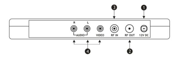
**Step 1:** Connect Female Connector of RF Cable provided to you, to **2** Connect the other end of cable (Male connector) to your Television Set. (The Female connector is present at the rear side of the TV).
